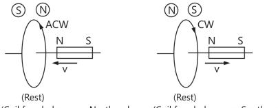
(Coil face behaves as North pole to oppose the motion of magnet)
